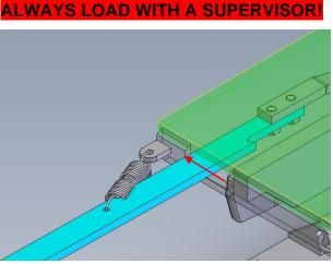
(The hitch plate hand leaver has to be at the limit in the direction of the spring)
