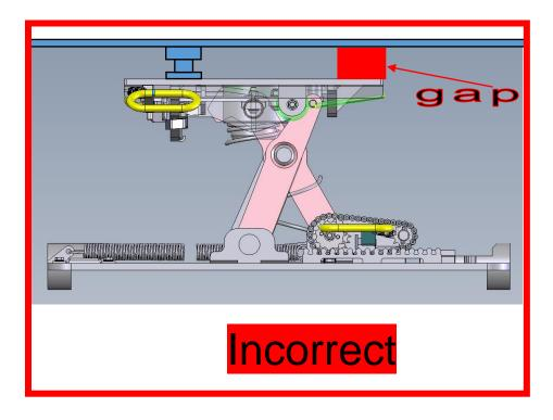
The king pin is correctly locked if the king pin lock release lever (hitch plate 70400; pos. 16 and 17) is at right angles to the hitch plate!
