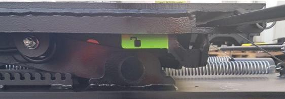
As long as the indicator (red or green > dependant on the customer) is visible, the king pin is not in the funnel. Not the indicator is not longer visible, is the kingpin situated in the funnel.
